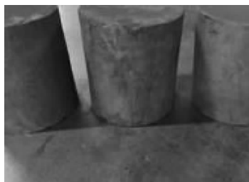
图 9 等静压成形的石墨生坯 Fig. 9 Graphite green billet formed by isostatic pressing
