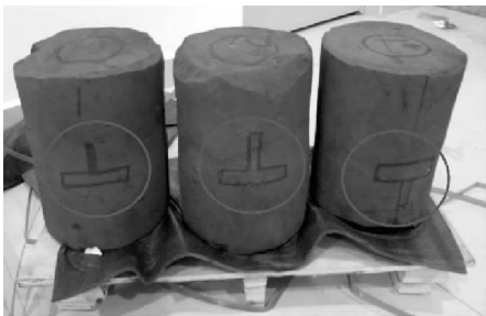
图 12 X 光标识石墨内部模板位置 Fig.12 Position of framework inside the graphite marked by X-ray
